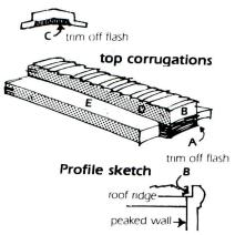
Due to mold and casting requirements, both ends of the roof ridge pieces have flash that must be trimmed away. Here is a simplified sketch of the roof ridge piece(s). (A) is white flash that must be trimmed away so that the end of the roof ridge piece (B) will rest on the inside "flange" of the peaked end walls. At the opposite end of the roof ridge there is also a piece of flash (C) that must be removed so that the roof ridge support
