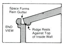
gap which forms the rain gutter. The other end butts up against (D) on the roof ridge sketch, and rests on (E).
